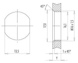
Installation direction: o-ring sits on chamfer.
